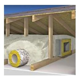
Also remember where at least 25% of a duct system or the air handler/furnace is located outside the thermal envelope, duct blaster testing is required.
